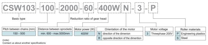
This is the geared motors. When you change the conveyance speed, you have to change all included motor. Contact us when distance between sprockets L is over 5000mm
